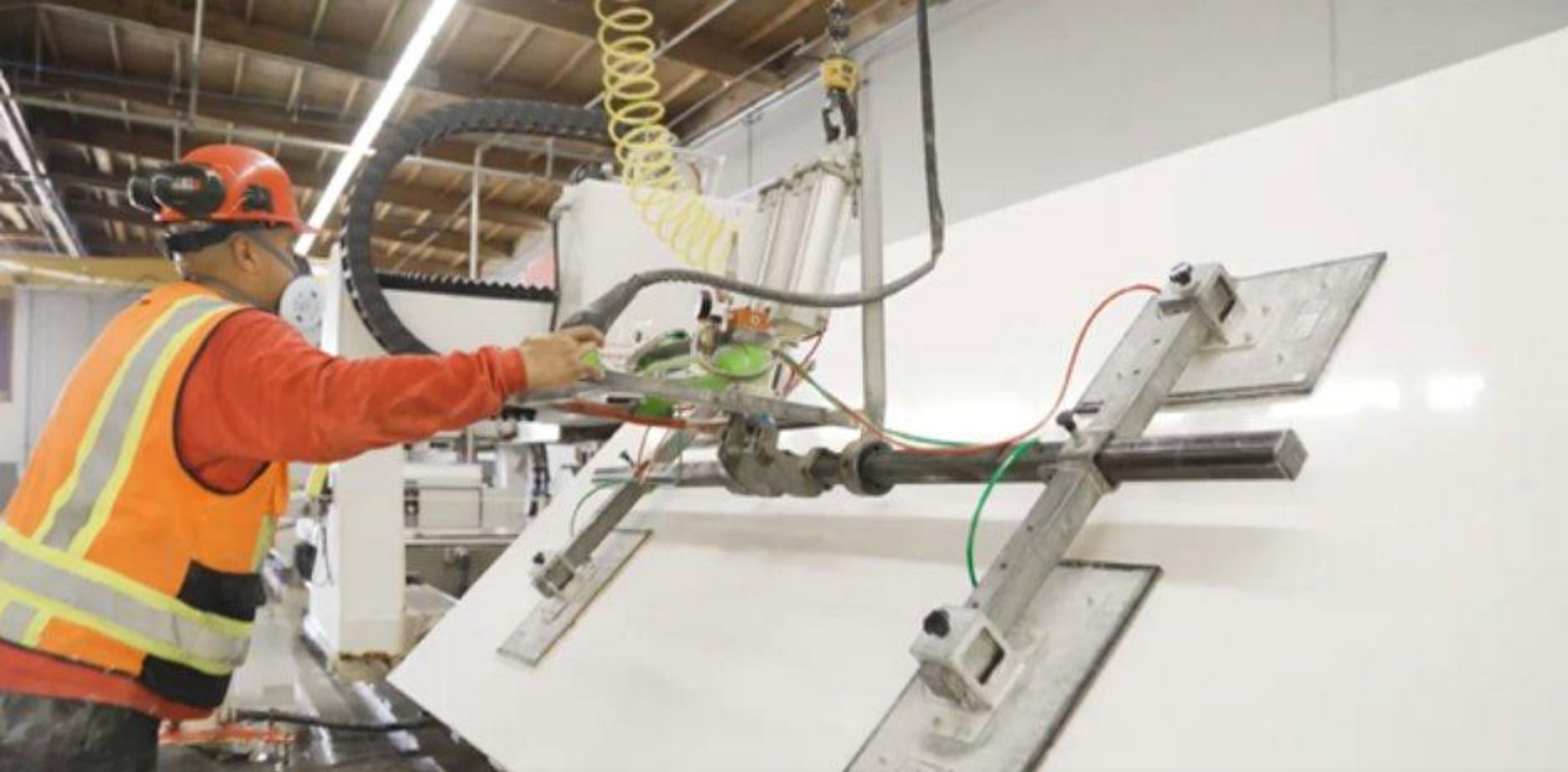
A CNC operator, affected worker of ASW, using a vacuum lifter system to load a slab of artificial stone equipped with PPE; engineering controls in use.
